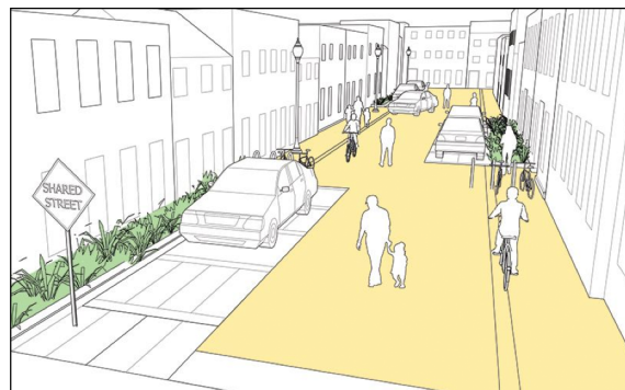
NACTO Shared Street Diagrams displaying how a typical street can be renovated into a shared street
