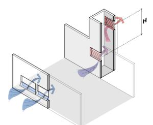
5. The *ventilation shaft height [H]* is measured from the center of the shaft intake to the center of the shaft outlet. The total amount of heat removed from a space is proportional to the height of the ventilation shaft. The higher the shaft, the greater the volume of air displaced.
