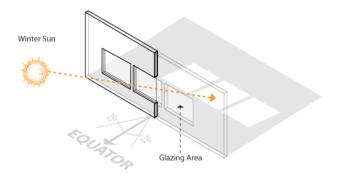
1. Direct Gain glazing can be integrated into the vertical skin of the solar façade — fixed or operable windows, glazed doors, and curtain walls.
