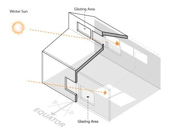
2. Direct Gain glazing can be integrated into a clerestory located on the solar façade (i.e. facing the equator). Clerestory glazing allows for additional freedom when locating spaces with exposure to the roof plane, and can reduce interior glare, provide privacy, and is less likely to be shaded by off-site obstructions.
