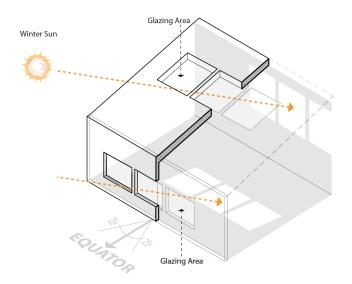
3. Direct Gain glazing can be integrated into a solar facing sloped skylight to admit sunlight through the roof of a space. As with clerestories, using skylights to provide top heating allows for additional freedom when locating spaces with exposure to the roof plane, and can reduce interior glare, provide privacy, and is less likely to be shaded by off-site obstructions.
