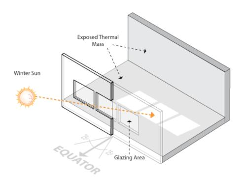
A Direct Gain passive heating system integrates the components of the system, solar glazing (solar collection) and thermal mass (heat storage medium), directly into a building. The most important factor in collecting the sun's energy is the placement and size of glazed openings.
